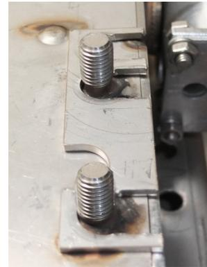
Abb. 8: Distanzblech (9) / pict. 8: spacing sheet (9)
