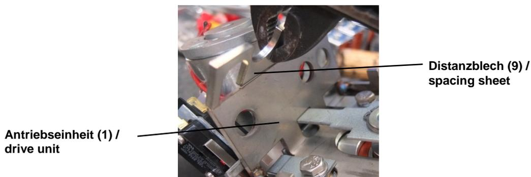
Abb. 7: Distanzblech / pict. 7: spacing sheet
